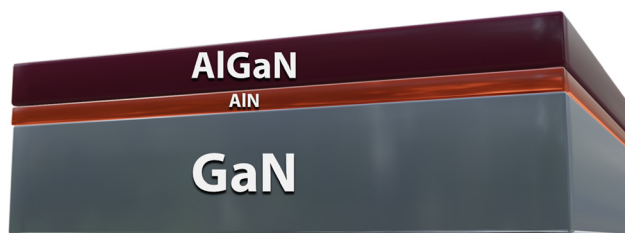
Fig. 1 Layout of the GaN/(AlN)/AlGaIn heterostructure grown by MOCVD on a sapphire substrate. From bottom to top: GaN buffer layer (blue), AlN interlayer (orange), and AlGaIn (purple). The nominal thickness of the AlN interlayer was: 0 nm (heterostructure A); 1.5 nm (heterostructure B); 3 nm (heterostructure C).
