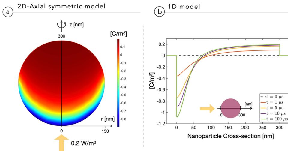
Fig. 2 Charge density distribution across the NP irradiated by a light intensity of  $0.2 \text{ W m}^{-2}$  impinging as depicted by the yellow arrow. (a) Results obtained using the 2DAS NP model. (b) Results obtained using the 1D-model as a function of time after the illumination.
