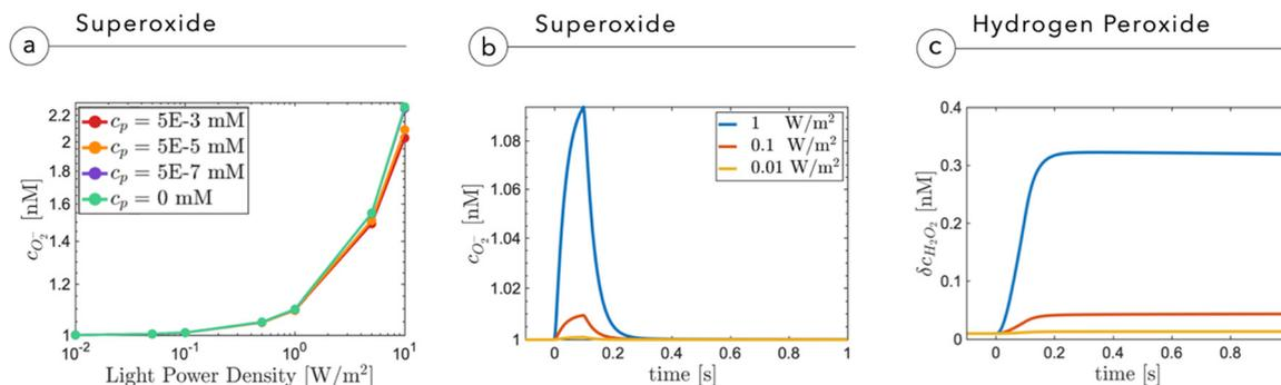
Fig. 5 (a) Superoxide concentration as a function of the protein concentration and the light intensity impinging onto the NP. (b) Profile of superoxide  $c_{O_2^-}(0^+, t)$  as a function of time at different light intensities. (c) Variation of hydrogen peroxide concentration  $\delta c_{H_2O_2}$  secondary to the production of superoxide.
