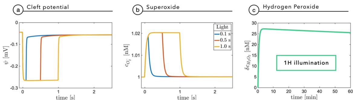
Fig. 6 Panels (a) and (b) show the simulation of the changes in the electric potential  $\psi(0, t)$  and the superoxide concentration in response to light stimuli at a power density of  $0.2 \text{ W m}^{-2}$  for increasing durations from 100 ms to 1 s. Panel (c) illustrates the variation of the hydrogen peroxide concentration with respect to its equilibrium value after one hour of illumination.
