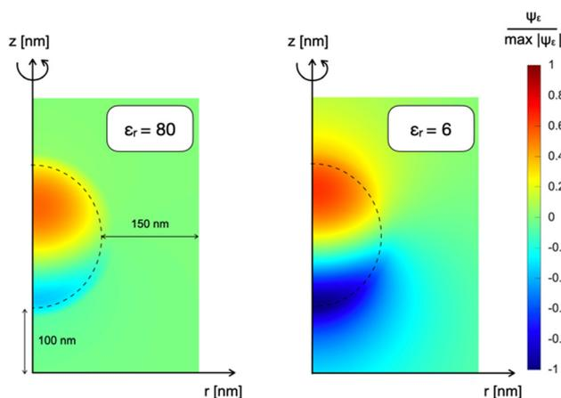
Fig. 3 Normalized electrostatic potential  $\Psi_\epsilon$  distribution of a NP immersed in an empty medium characterized by different dielectric constants: on the left  $\epsilon_r = 80$ ; on the right  $\epsilon_r = 6$ .
