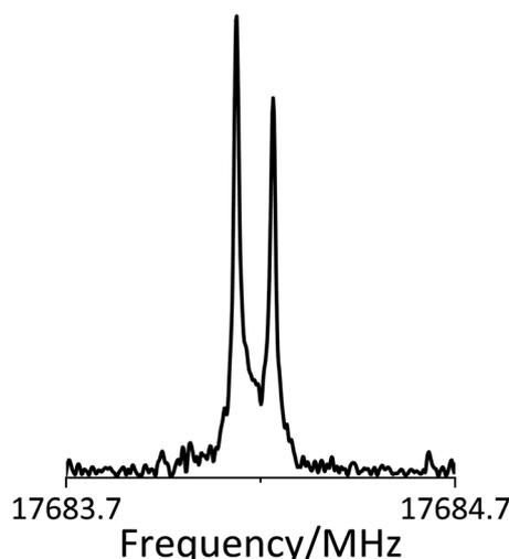
**Fig. 1** FTMW spectrum of the  $2_{11}-1_{10}$   $J = 2.5-1.5$   $F = 2.0-1.0$  transition. The spectrum is obtained by accumulating 100 shots of free induction decay signals. The spectral line shows the Doppler doubling due to the parallel orientation of the microwave and the jet propagations.
