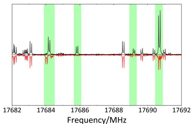
Fig. 2 Observed spectrum of  $^{35}\text{ClSO}$  for  $2_{11}-1_{10}$ . The upper trace (black) is that observed with the Earth's magnetic field compensation, while the lower trace (red) is that observed without the compensation. The marked spectral lines show the paramagnetic behavior, splitting or disappearance of the lines without the compensation.
