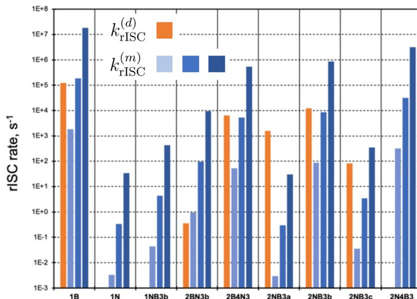
Fig. 4 Direct ( $d$ ) and mediated ( $m$ ) rate constants (in  $\text{s}^{-1}$ ) for molecules with  $|\Delta E_{ST}| < 0.5 \text{ eV}$ .  $k_{\text{rISC}}^{(m)}$  has been computed for weak (1 meV, light blue), medium (10 meV, blue), and strong (100 meV, dark blue) vibronic couplings, respectively. Intermediate values to compute direct and mediated rates can be found in Table S5 (ESI<sup>†</sup>).
