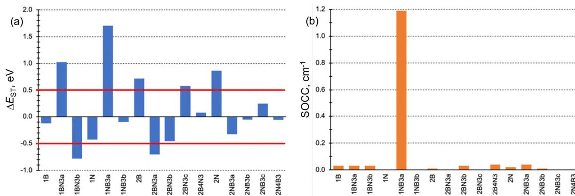
Fig. 3 (a) Excited singlet-triplet energy gaps ( $\Delta E_{ST}$  in eV) and (b) SOC constants (SOCC in  $\text{cm}^{-1}$ ) for the studied B and N doped phenalene and triangulene molecules.
