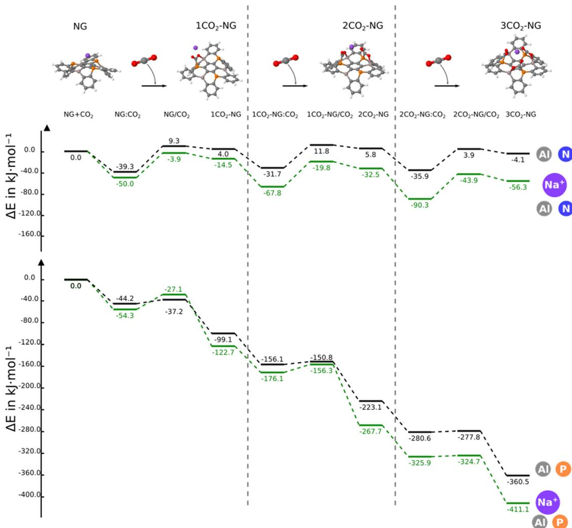
Fig. 8 Comparative energy profiles for the reaction of  $\text{Al}_3\text{N}_3\text{-NG}$  and  $\text{Al}_3\text{P}_3\text{-NG}$  in the absence/presence of  $\text{Na}^+$  with three  $\text{CO}_2$  molecules.
