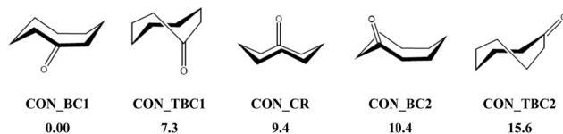
Scheme 2 Five low-energy CON conformers as reported in ref. 28. We have also given their relative energies (in \text{kJ mol}^{-1} ) with respect to the most stable one.
