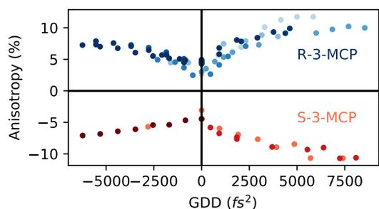
Fig. 6 Multiple anisotropy measurements as a function of chirp parameter at a central wavelength of 309 nm for (*R*)-(+)-3-MCP (shades of blue) and (*S*)-(-)-3-MCP (shades of red). Positive chirp leads to a larger enhancement of the anisotropy than negative chirp at this wavelength.
