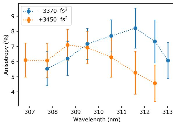
Fig. 8 Wavelength scan of the anisotropy of (*R*)-(+)-3-MCP at similar positive ( $+3450 \text{ fs}^2$ ) (in orange) and negative ( $-3370 \text{ fs}^2$ ) (in blue) linear chirp. The pulse energy was fixed for all measurements.
