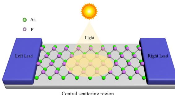
**Tunable electronic and optoelectronic characteristics of two-dimensional  $\beta$ -AsP monolayer: a first-principles study**
