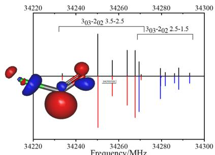
**Fourier-transform microwave spectroscopy of the ClCO radical**
