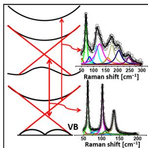
**Polarization-resolved resonant Raman excitation of surface and bulk electronic bands and phonons in MBE-grown topological insulator thin films**
