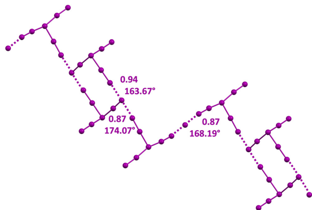
Fig. 6 Ball and stick representation of the infinite chain with pendants assembled via HaBs involving I^- and I_3^- anions in a salt of the tetrakis(10H)-phenothiazin-10-ium radical cation (Refcode EWEKUP). 108 Cations have been omitted for the sake of clarity; HaBs are violet dotted lines; HaB angles and Nc values are reported close to the interactions.
