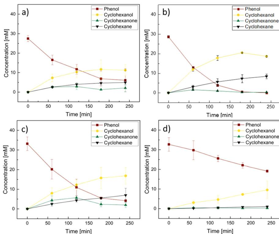
Fig. 6 Concentration profiles of phenol EC-HDO for a) comPtRu-C, b) labPtRu-C, c) Pt-C, and d) Ru-C (reaction conditions:  $50 \text{ mL min}^{-1} \text{ N}_2$ ,  $60^\circ \text{C}$ ,  $0.2 \text{ M}$  perchloric acid,  $0.2 \text{ mg cm}^{-2}$ , constant current  $55 \text{ mA cm}^{-2}$ ).
