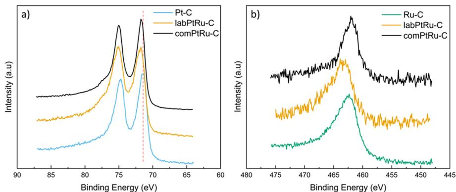
Fig. 5 XPS scans of the a) Pt 4f and b) Ru 3p binding energies for the comPtRu-C, labPtRu-C, Pt-C, and Ru-C. Dashed red line represents Pt(0) 4f<sub>7/2</sub> at 71.1 eV.
