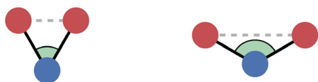
Fig. 6 Two different geometric graphs which are undistinguishable from distance edge features, but become distinguishable with angle information between edges or by adding the dashed edge to the graphs.
