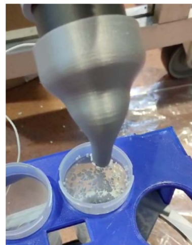
Fig. 11 Effect of static electricity in the working of the pellet distributor. Pellets can be seen getting attached to the cup walls and to the tip of the distributor. The aggregation of pellets inside the tube can cause a noticeably reduced throughput.
