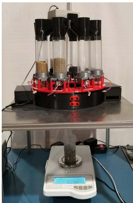
Fig. 4 Fully assembled dispenser placed on top of a table incorporating a funnel that directs the pellets to a plastic cup placed on a balance.
