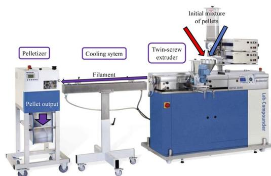
Fig. 1 Polymer extruder workflow illustrated by a Lab-Compounder KETSE 20/40, a water bath and a pelletizer, all of them from Brabender GmbH Co. KG.
