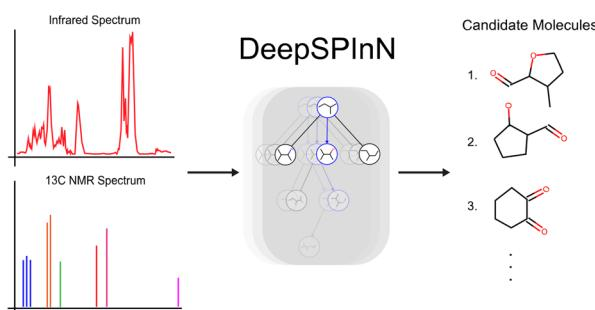
**DeepSPLnN – deep reinforcement learning for molecular structure prediction from infrared and  $^{13}\text{C}$  NMR spectra**
