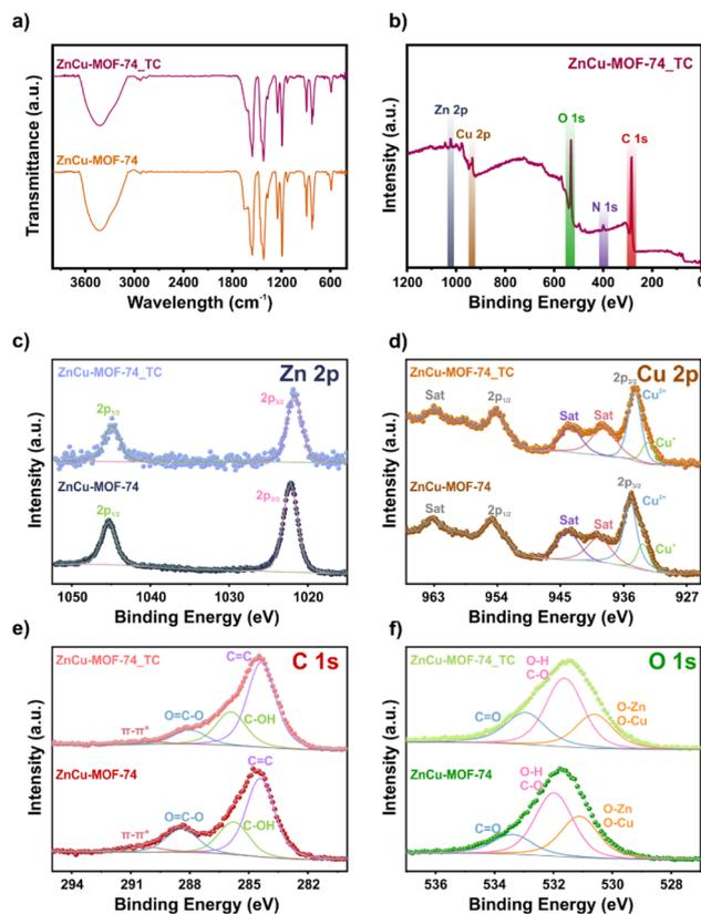
**Fig. 3** (a) FTIR before and after TC adsorption; (b) XPS survey spectrum of exhausted ZnCu-MOF-74; high-resolution spectra before and after TC adsorption of (c) Zn 2p, (d) Cu 2p, (e) C 1s, and (f) O 1s.
