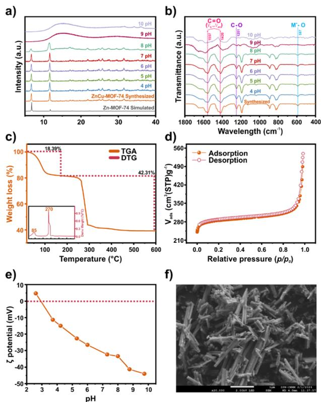
**Fig. 1** (a) PXRD diffractogram; (b) FT-IR spectra; (c) TGA–DTG analysis; (d) N<sub>2</sub> isotherm adsorption; (e) zeta potential; and (f) SEM micrographs of ZnCu-MOF-74 synthesized.
