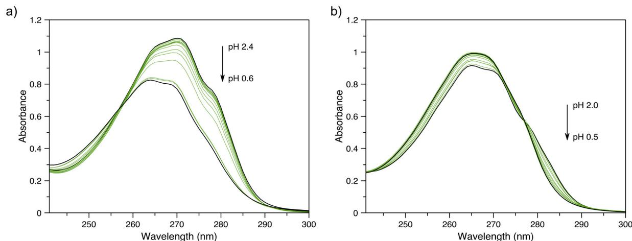
**Fig. 3** (a) Representative UV-vis spectra of solutions containing py-macrodipa and  $\text{InCl}_3$  in spectrophotometric titrations over the pH range of 0.6–2.4. (b) Representative UV-vis spectra of solutions containing py<sub>2</sub>-macrodipa and  $\text{InCl}_3$  in spectrophotometric titrations over the pH range 0.5–2.0.
