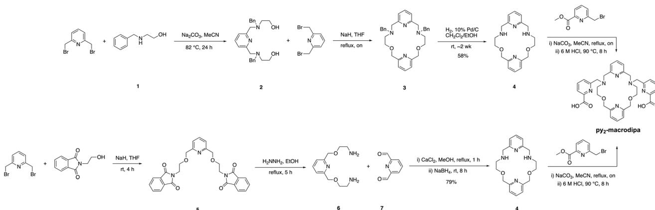
**Scheme 1** Previously reported synthetic approach of dipyridine macrocyclic backbone (top) and improved synthetic approach of dipyridine macrocyclic backbone by using metal ion template synthesis (bottom).
