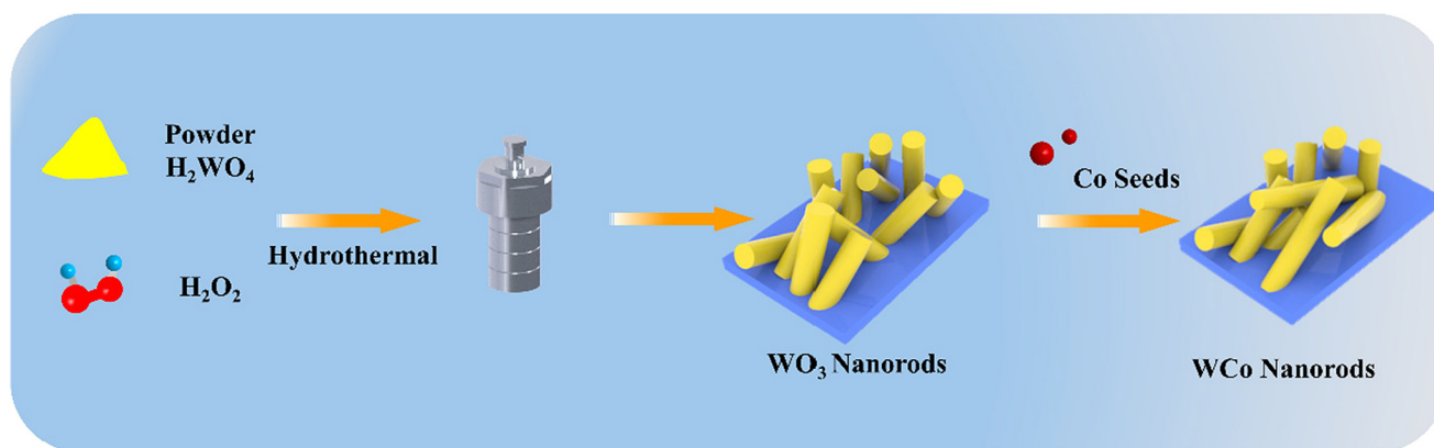
Fig. 1 Schematic diagram of the formation process of Co-doped \text{WO}_3 nanorods prepared by a hydrothermal method.
