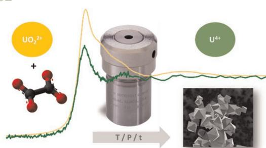
Reductive hydrothermal conversion of uranyl oxalates into UO<sub>2+x</sub> monitored by *in situ* XANES analyses
