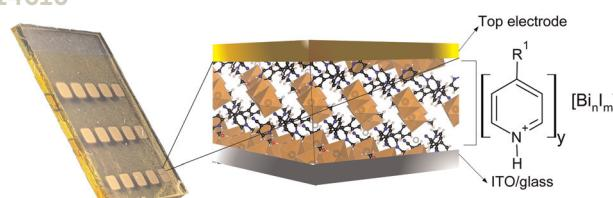
**Memristive properties and synaptic plasticity in substituted pyridinium iodobismuthates**
