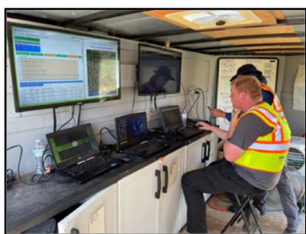
Fig. 14 Multi-vehicle telemetry base station and monitoring displays.
