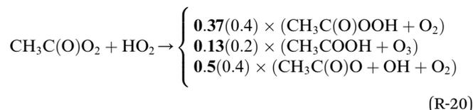
The reaction product CH<sub>3</sub>C(O)O decomposes into CO<sub>2</sub> and CH<sub>3</sub> and subsequent O<sub>2</sub> reaction produces CH<sub>3</sub>O<sub>2</sub>. Furthermore,
