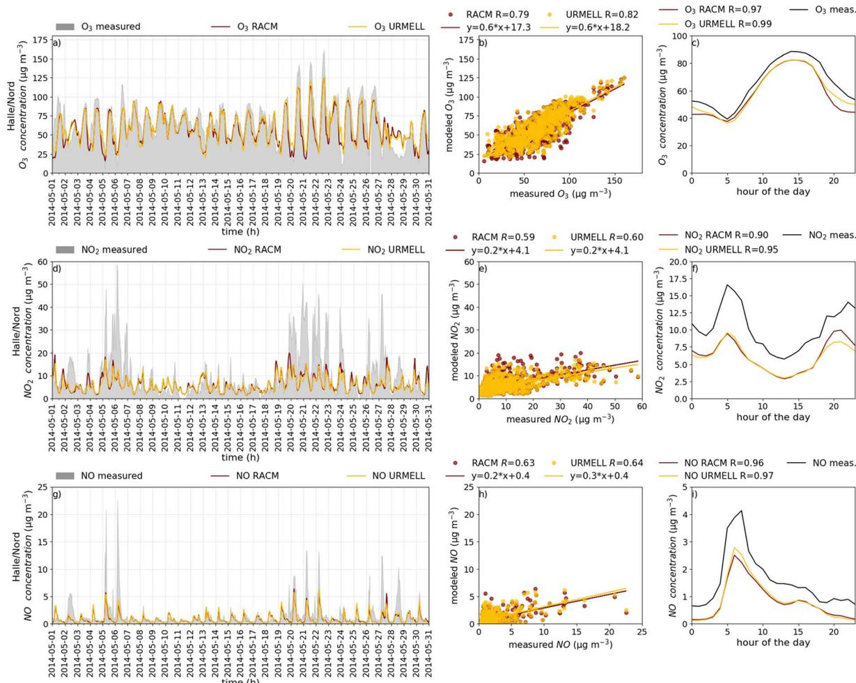
Fig. 5 Time series of O<sub>3</sub> in (a)–(c); of NO<sub>2</sub> in (d)–(f); of NO in (g)–(i) for Halle/Nord measurements in grey for (a), (d) and (g) black line otherwise as well as modeled concentrations using RACM (red line) and URMELL (yellow line).
