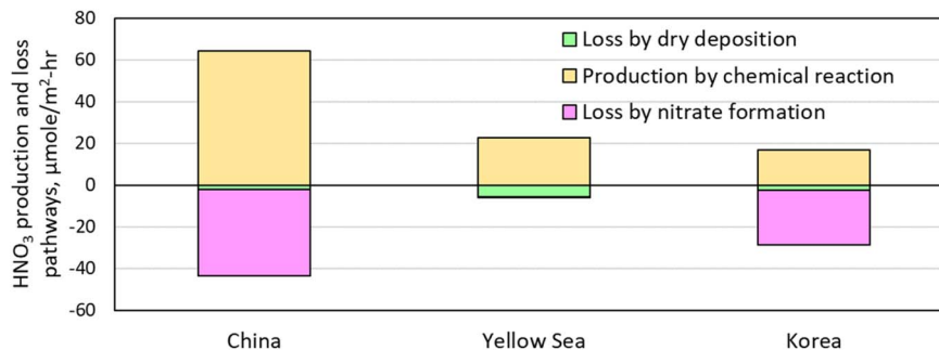
Fig. 11 HNO 3 chemical production rate, loss rates by dry deposition and nitrate formation in sub-areas of China, Yellow Sea, and Korea during the episode.
