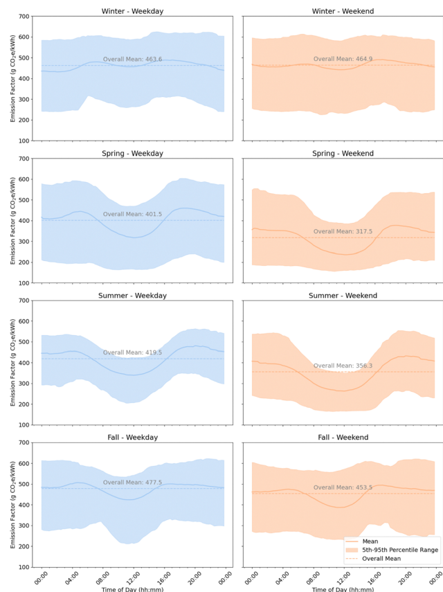
Fig. 8 Grid EF by day type, season, and time of day for the year 2021. The solid line represents the mean value for specific time points (e.g. 12:00 h), day type (e.g. weekday), and season (e.g. Summer). The shaded area delineates the range between the 5th and 95th percentiles of the data, highlighting the distribution's variability and indicating where 90% of the values lie for the given time and year. The dashed line represents the overall mean, i.e. , the daily mean for a given day type and season.
