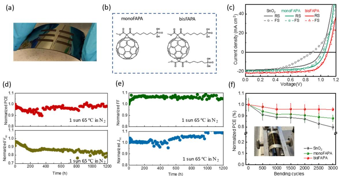
**Fig. 2** (a) Photograph of f-PSCs. (b) Chemical structures of monoFAPA and bisFAPA. (c) Representative  $J$ - $V$  curves measured with forward scanning (FS) and reverse scanning (RS) for reference and FAPA-modified devices. (d) and (e) Illumination stability under 1 sun and 65 °C in nitrogen atmosphere with bisFAPA modified device. (f) Normalized PCE of f-PSCs as a function of the number of mechanical bending cycles. The insert figure shows a photograph of the bending test.
