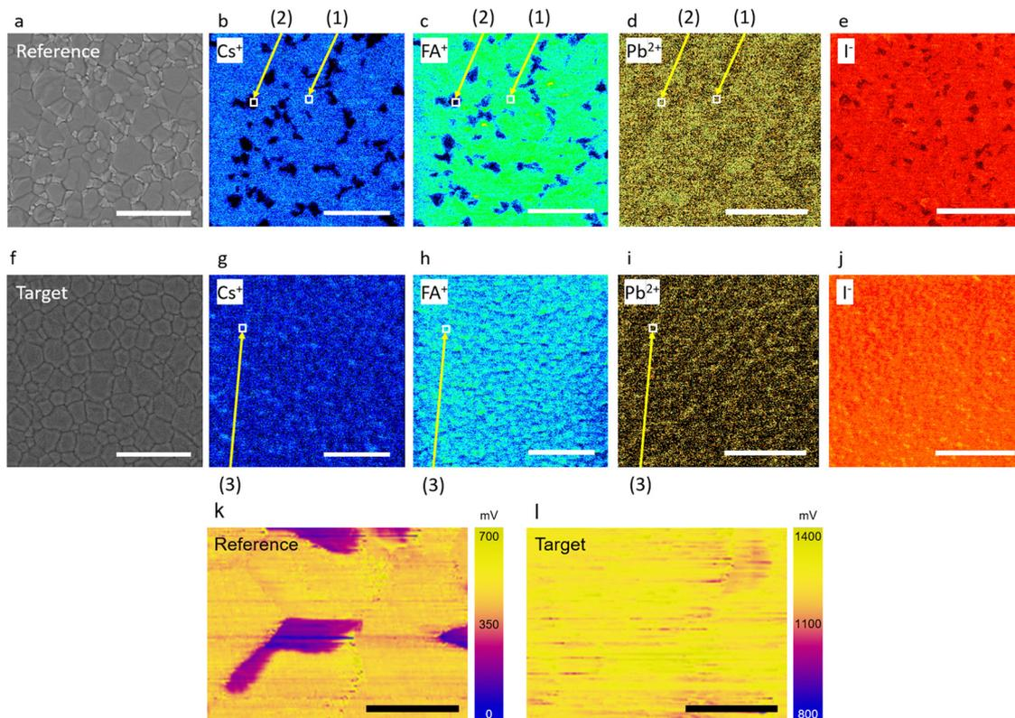
Fig. 2 HIM-SIMS and KPFM mapping of perovskite layers. Reference sample: (a) secondary electron image, SIMS mapping for (b) Cs<sup>+</sup>, (c) FA<sup>+</sup>, (d) Pb<sup>2+</sup>, and (e) I<sup>-</sup>. Target sample: (f) secondary electron image, SIMS mapping for (g) Cs<sup>+</sup>, (h) FA<sup>+</sup>, (i) Pb<sup>2+</sup>, and (j) I<sup>-</sup>, scale bar is 5 μm. Surface potential of perovskite surface from KPFM for (k) reference and (l) target, scale bar is 1 μm.
