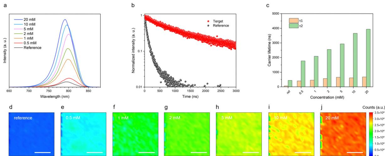
**Fig. 3** Photoluminescence spectroscopy of the perovskite films. (a) Steady-state photoluminescence emission (PL emission) spectra, (b) time-resolved photoluminescence (tr-PL) of the reference (without [N4444][TFSI]) and target (5 mM of [N4444][TFSI]), (c) carrier lifetime, and (d)–(j) photoluminescence mapping (PL mapping) of the perovskite films with 0, 0.5, 1, 2, 5, 10, and 20 mM concentrations of [N4444][TFSI] in the perovskite precursor solution. Scale bar is 200  $\mu\text{m}$ .
