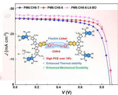
**Rational design of flexible-linked 3D dimeric acceptors for stable organic solar cells demonstrating 19.2% efficiency**
