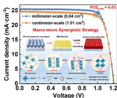
**Macro–micro coordination optimization of lead iodide reactivity toward millimeter-to-centimeter-scale perovskite solar cells with minimal efficiency loss**
