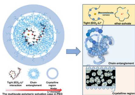
**The deconstruction of a polymeric solvation cage: a critical promotion strategy for PEO-based all-solid polymer electrolytes**
