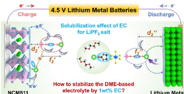
**Trace ethylene carbonate-mediated low-concentration ether-based electrolytes for high-voltage lithium metal batteries**
