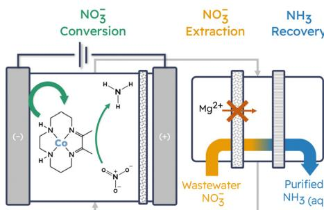
**Engineering a molecular electrocatalytic system for energy-efficient ammonia production from wastewater nitrate**
