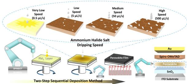
**Precise control of process parameters for <23% efficiency perovskite solar cells in ambient air using an automated device acceleration platform**
