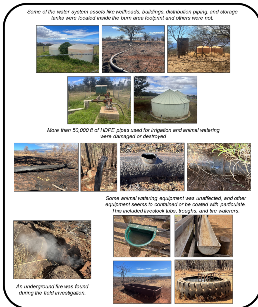
Fig. 3 Some agricultural water system assets were thermally damaged, destroyed, or impacted by particulate.
