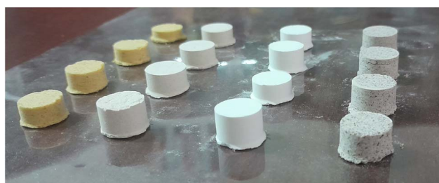
Fig. 3 The compacted dry flour samples of corn, wheat, barley and ragi (from left to right).
