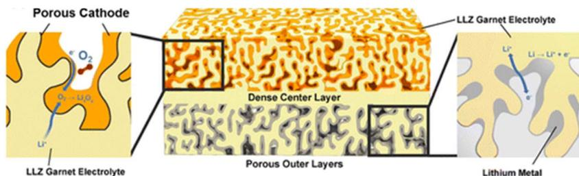
Fig. 4 Concept of a tri-layer garnet  $\text{Li}_7\text{La}_3\text{Zr}_2\text{O}_{12}$  (LLZ)  $\text{Li}-\text{O}_2$  cell with high interfacial surface area, short lithium-ion conduction pathways and minimized use of electrolyte material, taken from <https://doi.org/10.1039/D3FD00119A>.
