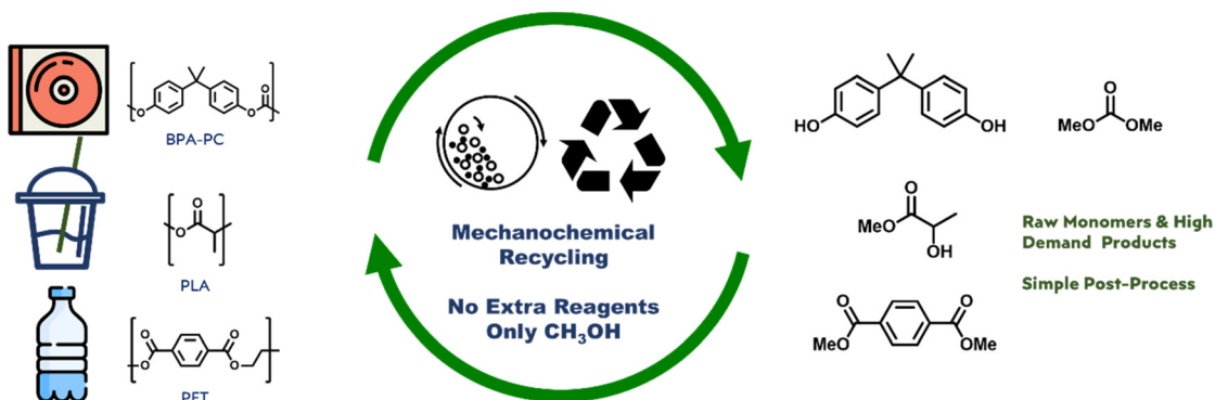
Fig. 1 Concept of mechanochemical recycling methanolysis of carbonate & ester plastics: no catalyst, no solvent, and high efficiency.
