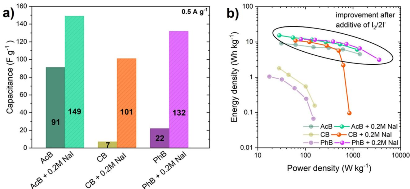
**Fig. 3** (a) Specific capacitance values at  $0.5 \text{ A g}^{-1}$  and (b) Ragone plots for ECs operating in acetate buffer, citrate buffer, and phosphate buffer with/without  $0.2 \text{ mol L}^{-1}$  NaI additive.
