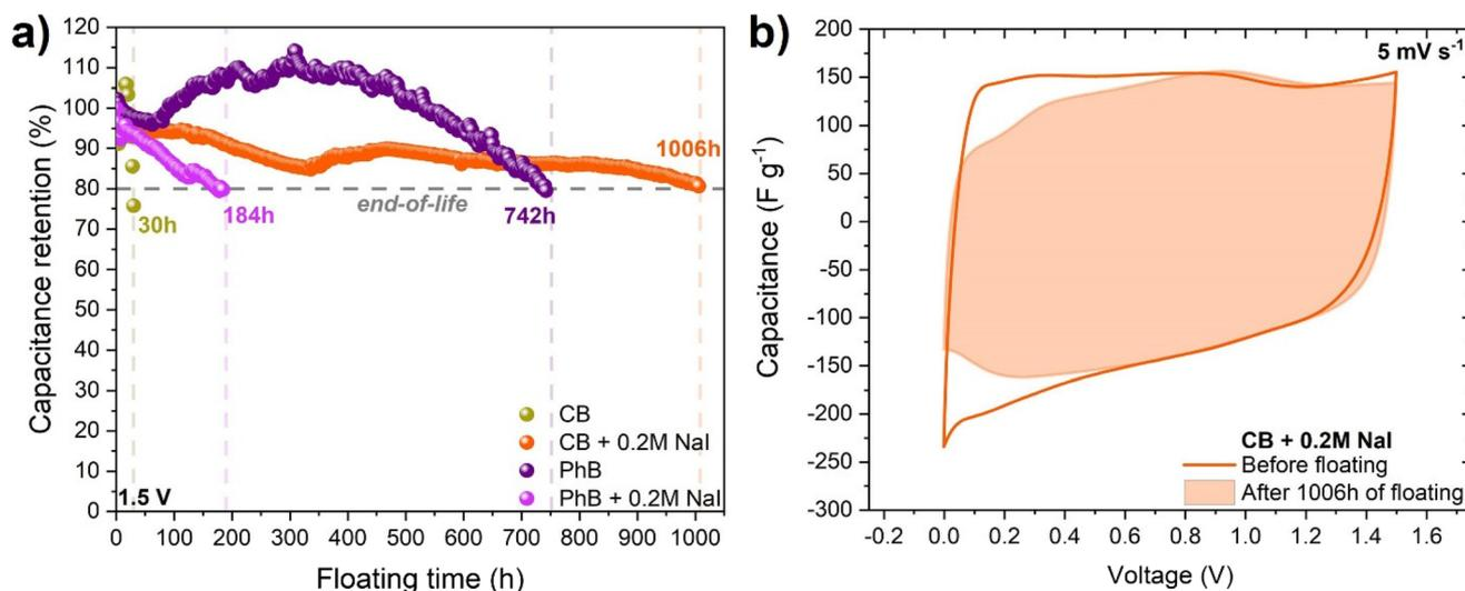
Fig. 5 (a) Capacitance retention of YP50F-based ECs operating in citrate buffer and phosphate buffer with/without 0.2 mol L<sup>-1</sup> NaI additive during floating test (at 1.5 V). Cyclic voltammograms for ECs operating in (b) citrate buffer + 0.2 mol L<sup>-1</sup> NaI before and after 1006 h floating test.
