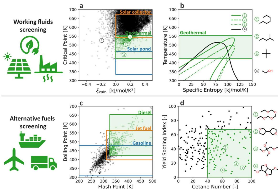
**Fig. 8** Application of the GAT model for working fluid and alternative fuels screening. (a) Distribution of ~27 000 organic molecules on  $T_c$ - $\xi$  axis, (b)  $T$ - $s$  curve of four different working fluids with varying  $T_c$  and  $\xi$ , (c) distribution of ~1300 saturated ethers on  $T_B$ -FP axis, and (d) sub-screening based on YSI and CN.
