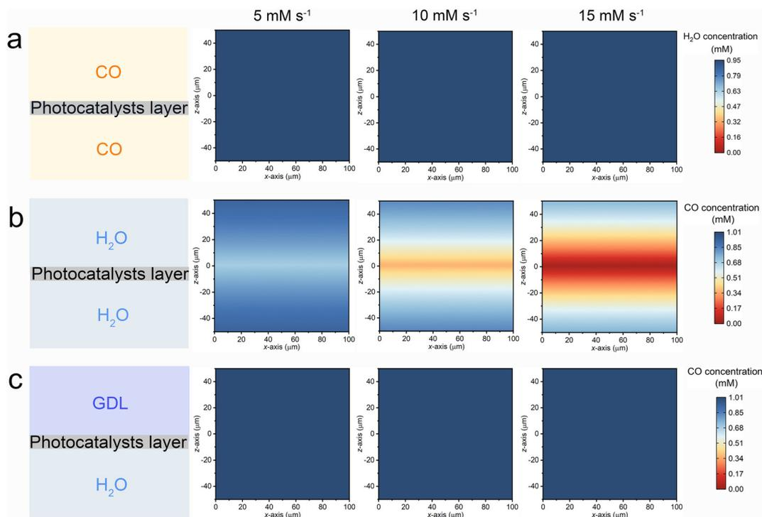
**Fig. 5** Schematic diagrams and FEM simulation results of (a) G–S, (b) L–S, and (c) G–L–S systems. The colour scale in (a) represents the water vapor concentration, in (b) and (c) represents the CO concentration.
