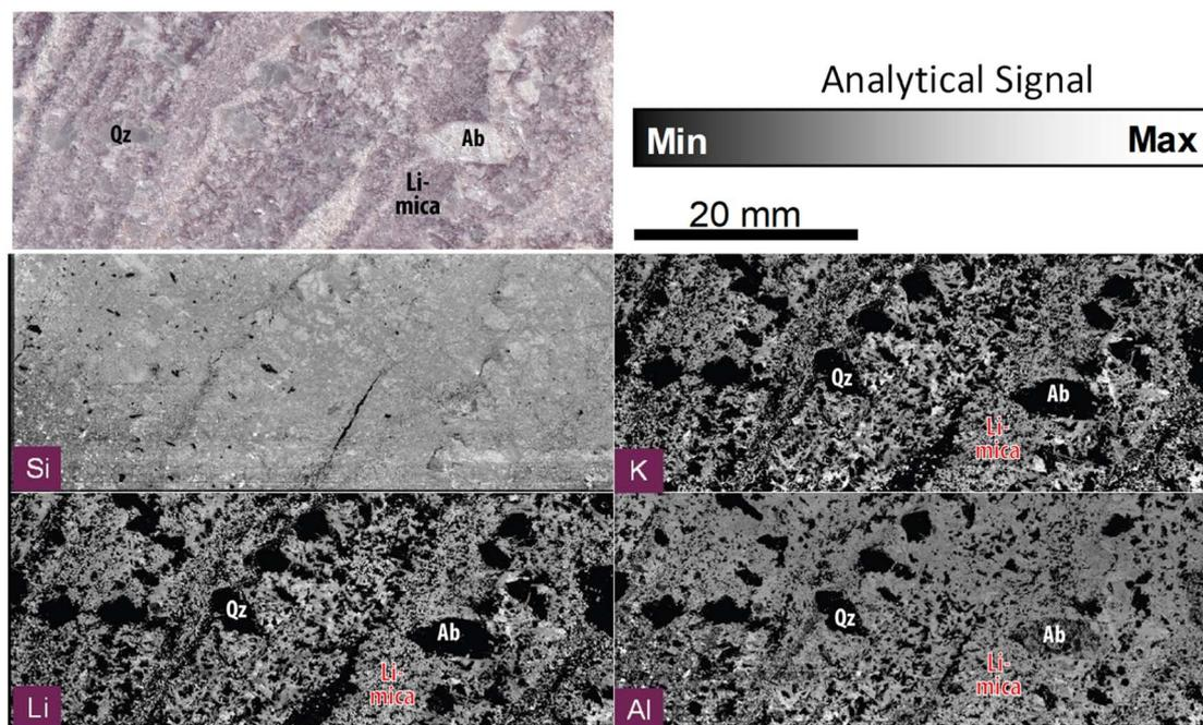
Fig. 2 Compositional imaging using the analytical signal for the emission lines of Si  $I_{288\text{ nm}}$ , K  $I_{766\text{ nm}}$ , Li  $I_{670\text{ nm}}$  and Al  $I_{308\text{ nm}}$ , and the optical picture of the Almendra's sample.
