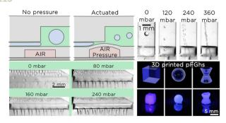
Tuna-step: tunable parallelized step emulsification for the generation of droplets with dynamic volume control to 3D print functionally graded porous materials
