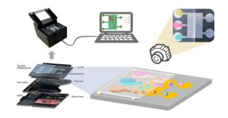
Measuring the electrophoretic mobility and size of single particles using microfluidic transverse AC electrophoresis (TrACE)
