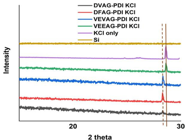
Fig. 1 XRD scans of fresh samples show formation of KCl for  $\pi$ -peptide/KCl hybrid structures. DVAG, DFAG, and VEVAG show lattice spacing increases from about 3.11 to 3.17 angstroms, and the peak positions are consistent with the (200) peak of KCl, though the three bottom traces can be slightly different polymorphs.
