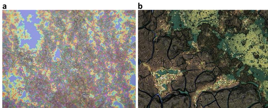
**Fig. 7** (a) 50 $\times$  micrograph of templated CdS growth from self-assembling DFAG peptides with 0.01 M CdA, and thioacetamide. (DFAG 0.01 M CdS) (b) 50 $\times$  micrograph of CdS grown from self-assembling DFAG peptides with 1 M CdA, and thioacetamide. (DFAG 1 M CdS).
