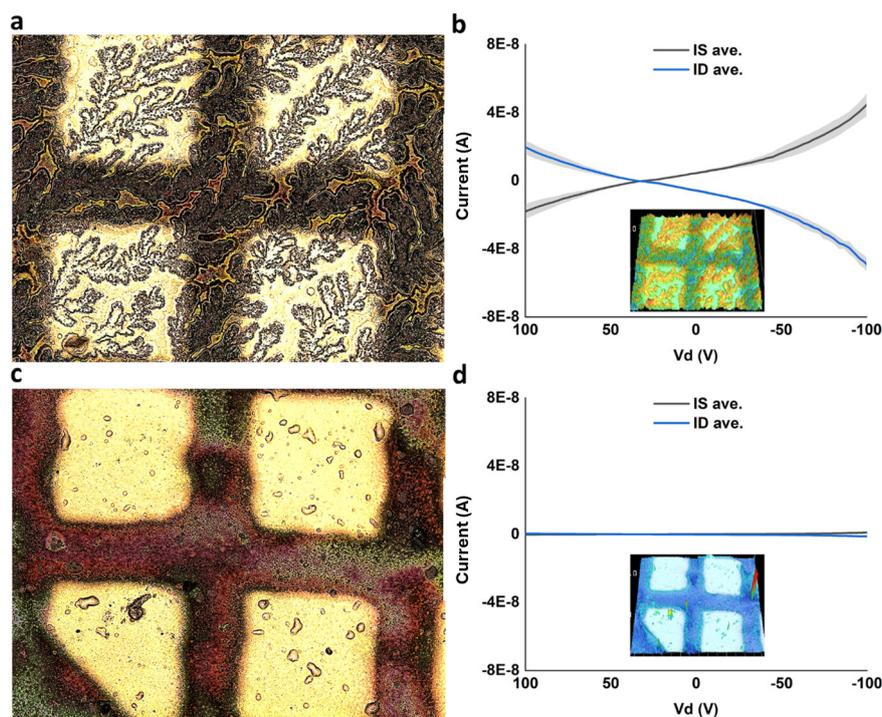
**Fig. 10** (a) Highly dendritic regions of VEEAG-PDI/CsCl with thermally evaporated Au electrodes. (b) Electrical measurements of dendritic region showed notable conductivity. (c) Blank regions of VEEAG-PDI/CsCl with thermally evaporated Au electrodes. (d) Electrical measurements of blank region showed no conductivity. Insets at (b) and (d) show 3D height scan of electrodes measured.
