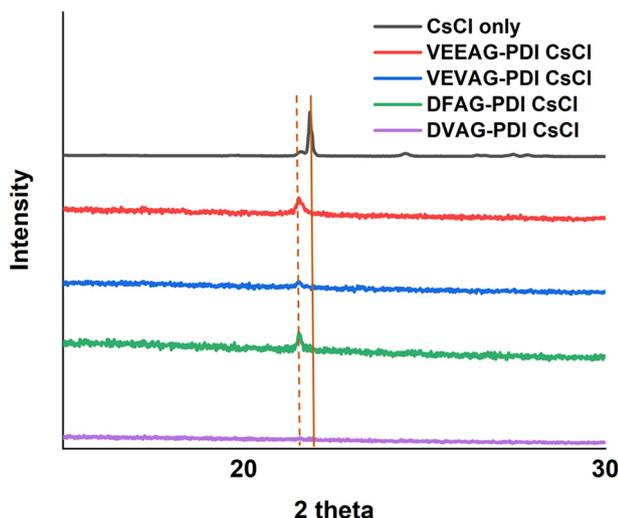
Fig. 2 XRD scans show formation of CsCl for  $\pi$ -peptide/CsCl hybrid structures. The peak position is consistent with a published diffractogram.<sup>59</sup>
