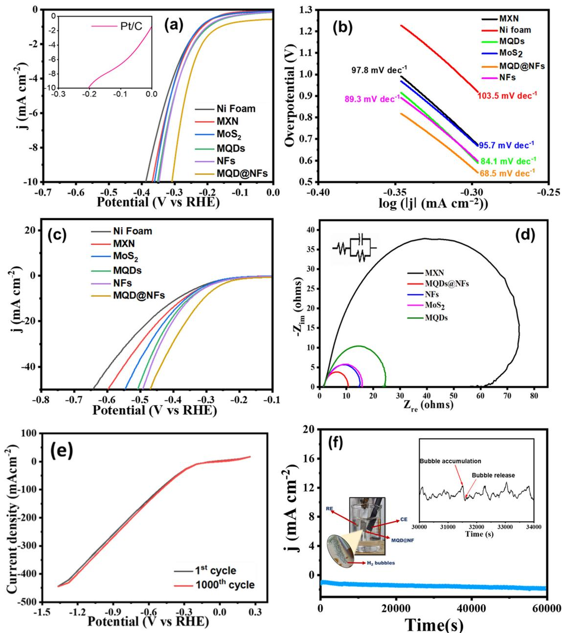
Fig. 7 (a) LSV, (b) Tafel plot, (c) LSV at high current density, (d) impedance, (e) 1000 CV cycles, and (f) stability of MQD@NFs.
