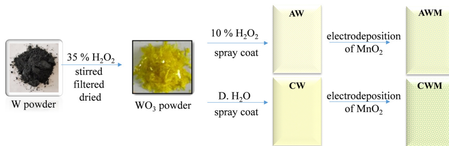
Fig. 1 Schematic representation of the fabrication process of MnO 2 coated WO 3 thin film electrodes.
