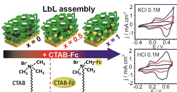
**Ferrocene-labelled surfactants enhance the supercapacitor performance in PANI-PSS/nanocarbon layer-by-layer nanoarchitectonics electrodes**
