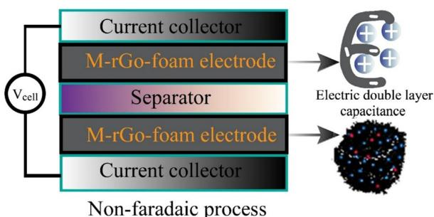
**A metallated graphene oxide foam with a carbon nanotube shell for an enhanced capacitance device**
