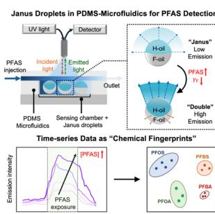
**Real-time detection and classification of PFAS using dynamic behaviors at liquid–liquid interfaces**
