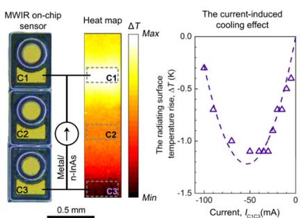
**Current induced cooling in a metal/n-InAs structure**
