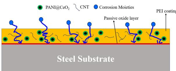
**A ‘tortuous path’ and ‘protective oxide layer’ work in tandem in unique corrosion-resistant polyetherimide coatings**
