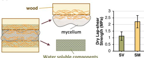
**A closer examination of white-rot fungal mycelia assisted wood bonding**
