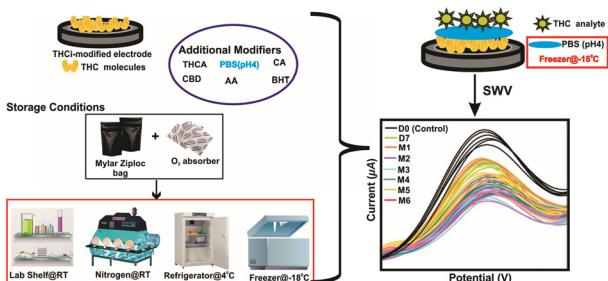
**Tetrahydrocannabinol (THC)-modified screen-printed carbon electrodes (SPCEs): insights into stability**
