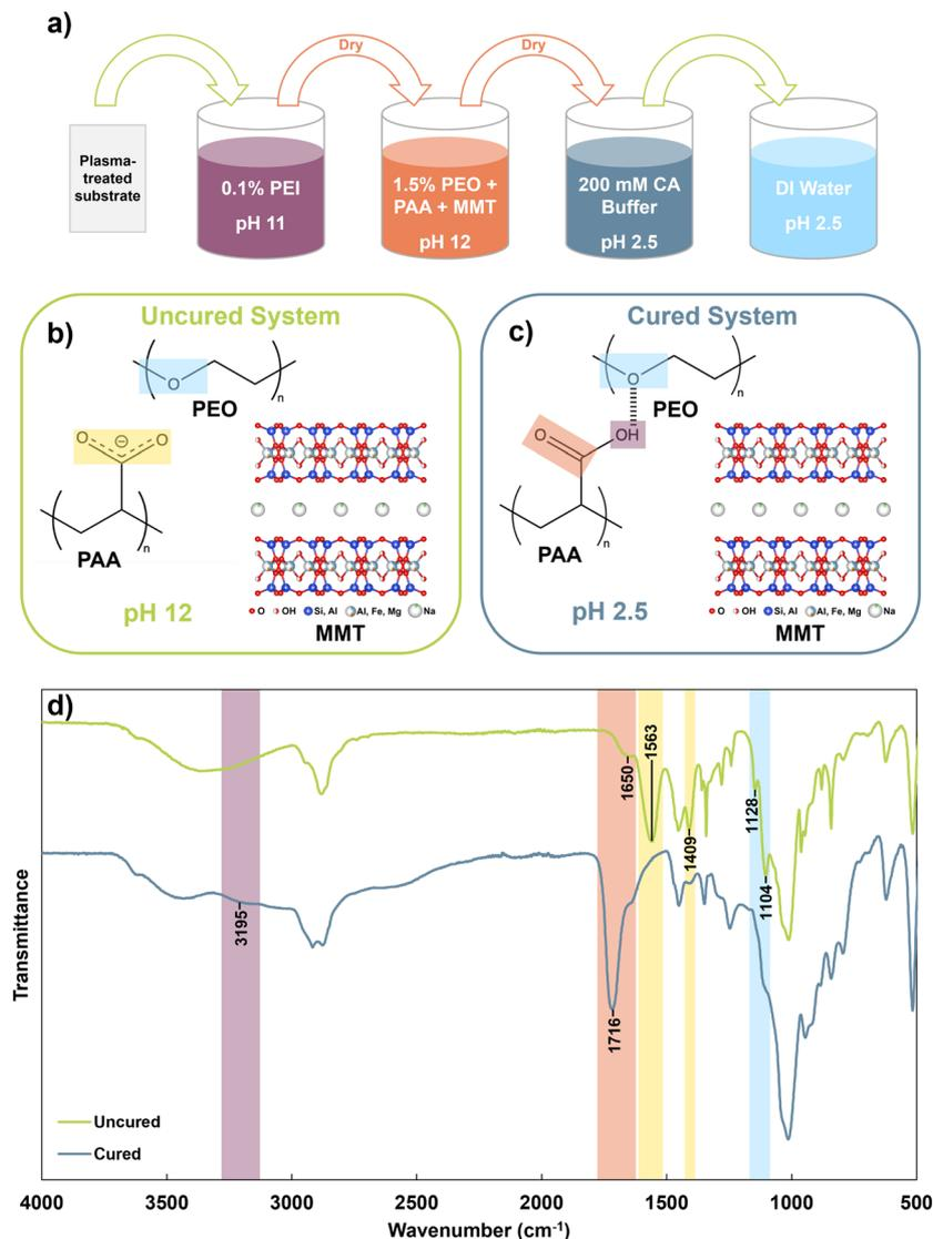
**Fig. 1** (a) Schematic of the HBPC coating process, (b) chemical structures of materials in coating solution, (c) chemical structures of materials in the cured coating, and (d) FTIR spectra of cured and uncured PPM 2 : 1 coatings, with key peaks labelled.
