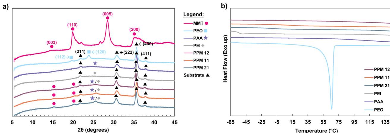
Fig. 3 (a) XRD spectra of coating components and PPM recipes and (b) DSC thermograms of coating components and PPM complexes.
