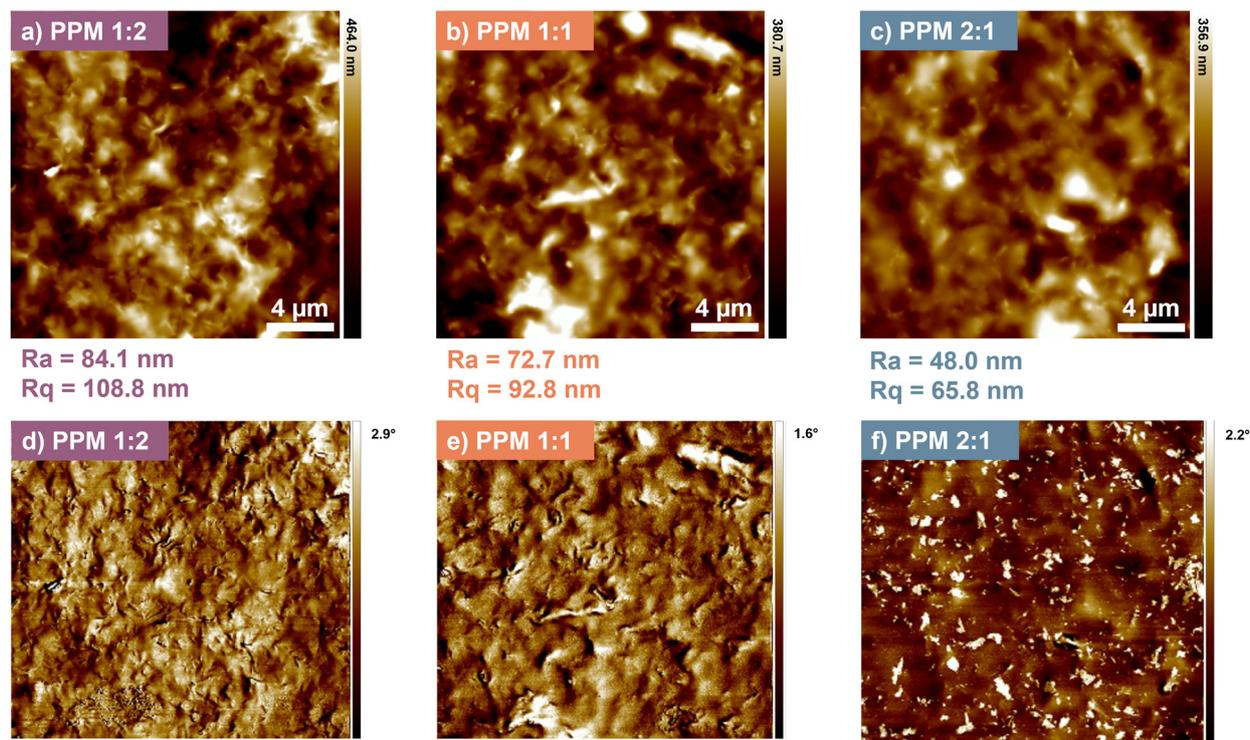
Fig. 5 AFM height images (a–c) and phase images (d–f) of PPM 1 : 2 (a and d), PPM 1 : 1 (b and e), and PPM 2 : 1 (c and f), including average roughness ( $R_a$ ) and root-mean-square roughness ( $R_q$ ) values.
