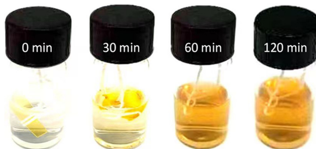
Fig. 9 Degradation process of VTICO-IPDI at different times in a 1 M HCl H 2 O/HFP (1/9, v/v) solution.
