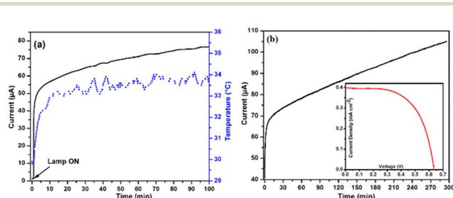
**Fig. 8**  $I$  vs.  $T$  measurement at (a)  $30 \text{ mW cm}^{-2}$  with temperature monitoring for 100 min and (b)  $40 \text{ mW cm}^{-2}$  for 300 min. (Inset)  $J$ - $V$  characteristics after 300 min of illumination.
