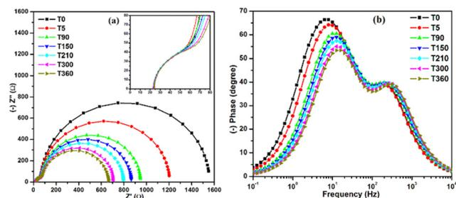
**Fig. 7** Device exposed to LED lamp at  $40 \text{ mW cm}^{-2}$ . (a) Impedance analysis at various time intervals; (inset) expanded initial region. (b) Bode plot derived from impedance analysis.
