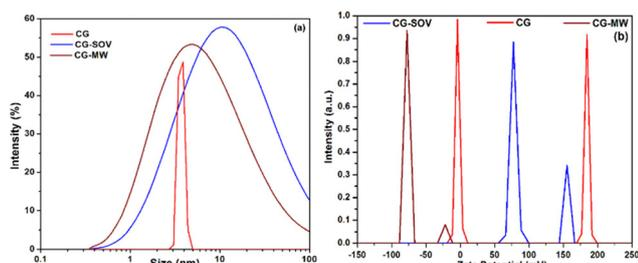
Fig. 5 (a) DLS measurement and (b) zeta potential of the CD.
