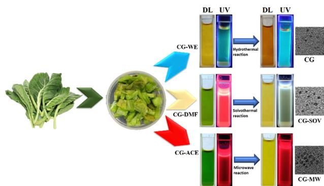
**Fig. 1** A schematic representation of the collard green CD synthesis. CG-WE stands for collard greens extract in water and ethanol solvent, CG-DMF stands for collard greens extract in DMF solvent and CG-ACE stands for collard greens extract in acetone solvent while CG, CG-SOV, and CG-MW are their corresponding CDs prepared by hydrothermal, solvothermal and microwave methods, respectively. DL: daylight; UV: ultra-violet light.
