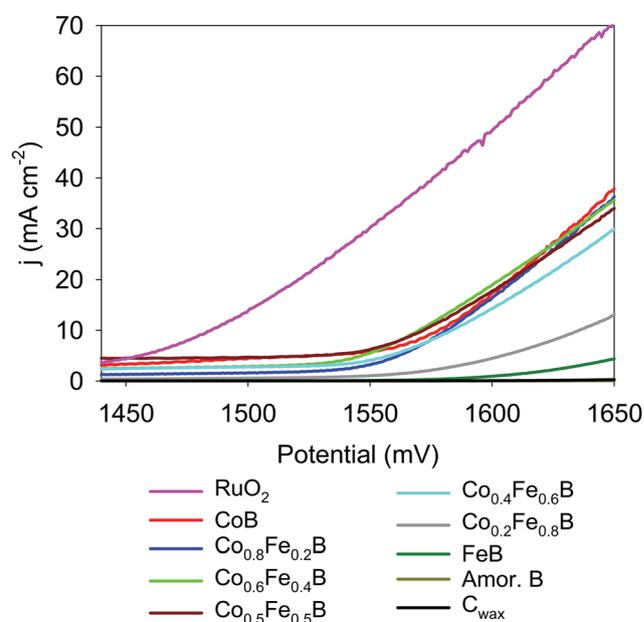
Fig. 8 Representative OER LSV results of CoB, FeB, and Co<sub>1-x</sub>Fe<sub>x</sub>B solid-solutions. Plots for the C<sub>wax</sub> and boron are shown for comparison. Data was obtained in O<sub>2</sub> purged 1.0 M KOH in a three-electrode cell at 5 mV s<sup>-1</sup> scan rate with Hg/HgO reference and graphite rod counter electrodes. Current densities are scaled using the geometric electrode area (0.08 cm<sup>2</sup>). Amorphous boron and C<sub>wax</sub> data are at baseline levels.
