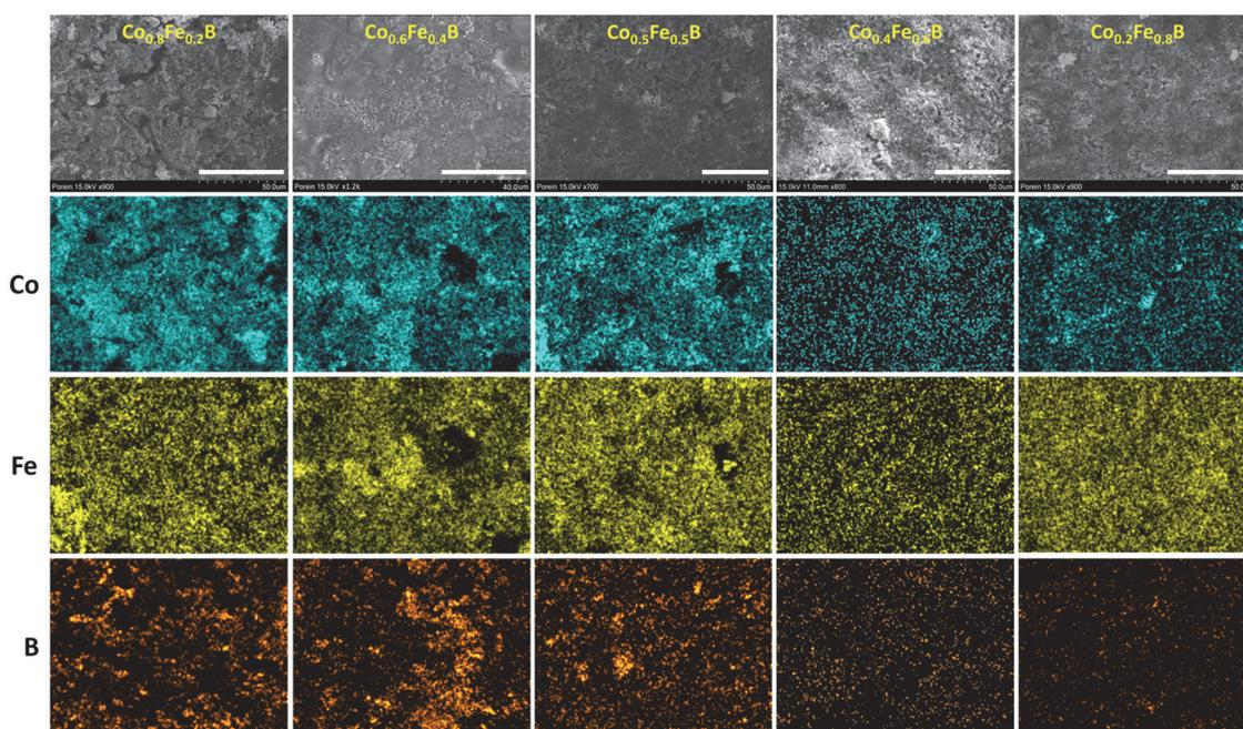
Fig. 5 EDS elemental mapping images of  $\text{Co}_{1-x}\text{Fe}_x\text{B}$  solid-solutions showing the transition from cobalt-rich to iron-rich products (left to right). The white scale bar in the SEM images is 40  $\mu\text{m}$  for  $\text{Co}_{0.6}\text{Fe}_{0.4}\text{B}$  and 50  $\mu\text{m}$  for other solid-solutions.
