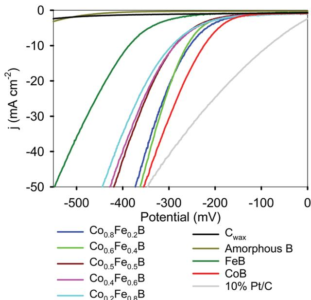
Fig. 7 Representative HER LSV results of CoB, FeB, and  $\text{Co}_{1-x}\text{Fe}_x\text{B}$  solid-solutions. Plots for the  $C_{\text{wax}}$  and amorphous B are shown for comparison. Data was obtained using 1.0 M KOH in a three-electrode cell at  $5 \text{ mV s}^{-1}$  scan rate with Hg/HgO reference and graphite rod counter electrodes. Current densities are scaled using the geometric electrode area ( $0.08 \text{ cm}^2$ ).
