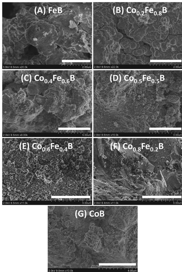
Fig. 6 Comparison of SEM particle morphologies for CoB, FeB and  $\text{Co}_{1-x}\text{Fe}_x\text{B}$  solid-solutions. Scale bar lengths are: (A) 2  $\mu\text{m}$ , (B) 2  $\mu\text{m}$ , (C) 5  $\mu\text{m}$ , (D) 3  $\mu\text{m}$ , (E) 5  $\mu\text{m}$ , (F) 5  $\mu\text{m}$ , (G) 4  $\mu\text{m}$ .
