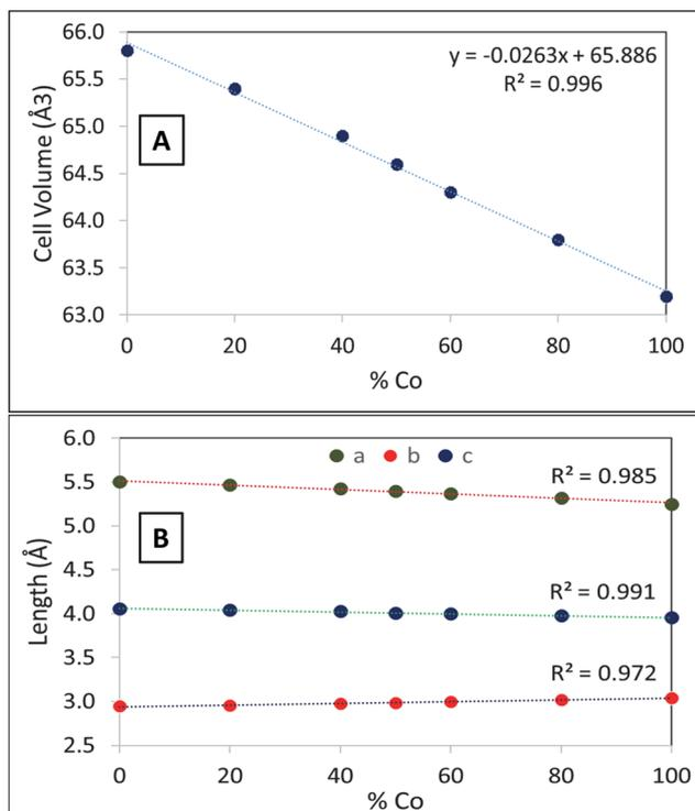
Fig. 4 Ideal percent Co in  $\text{Co}_{1-x}\text{Fe}_x\text{B}$  versus (A) unit cell volume, (B) unit cell parameters ( $a$ ,  $b$ ,  $c$ ). Linear regression lines for each data set are shown as dashed lines.
