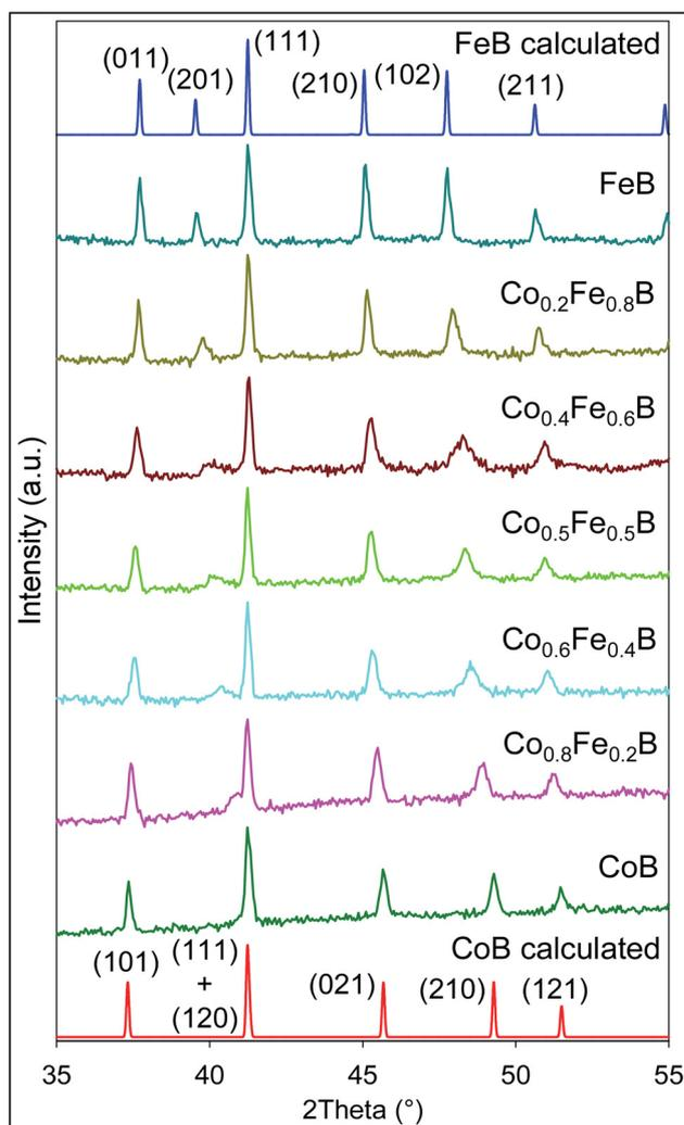
Fig. 3 Powder XRD stack plot of orthorhombic CoB, FeB, and  $Co_{1-x}Fe_xB$  solid solutions. Miller indices (*hkl*) are listed for FeB and CoB end members.
