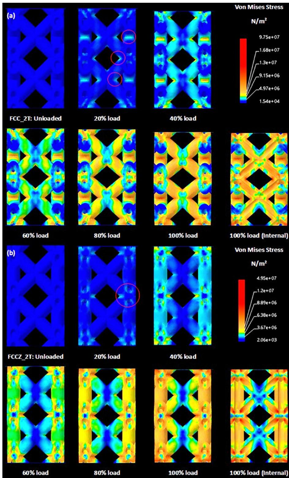
Fig. 12 Isotropic elastic continuum material FE model of double border scan (a) FCC, and (b) FCCZ unit cell responses to uniaxial compression in a  $2 \times 2 \times 1$  lattice array under varying loading conditions.
