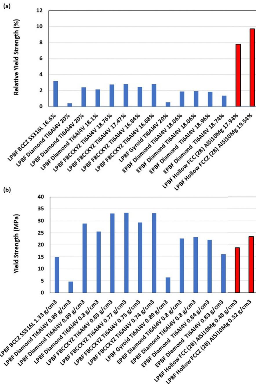
Fig. 8 Comparison of relative yield strength (a) and absolute yield strength (b) between FCC<sub>2B</sub> and FCCZ<sub>2B</sub> AlSi10Mg hollow-strut lattices and Ti-6Al-4V and SS316L solid-strut lattices of similar relative density (17–20%).<sup>53,54,78–82</sup> The name of each data point on the X-axis denotes “unit cell topology, material, relative or absolute density”. Error bars were not included as the standard deviation between samples was negligible.
