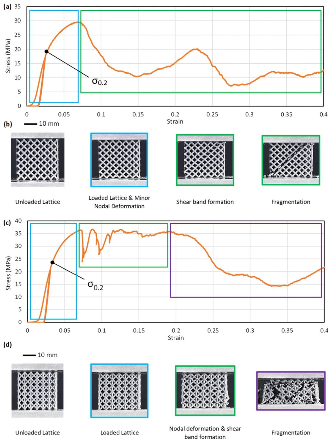
**Fig. 9** Failure modes and stress–strain curves. (a) The stress–strain curve for FCC\_2B AlSi10Mg hollow-strut lattices. (b) Photos of lattice specimens corresponding to different deformation stages in (a). (c) The stress–strain curve for FCCZ\_2B AlSi10Mg hollow-strut lattices. (d) Photos of lattice specimens corresponding to different deformation stages in (c).
