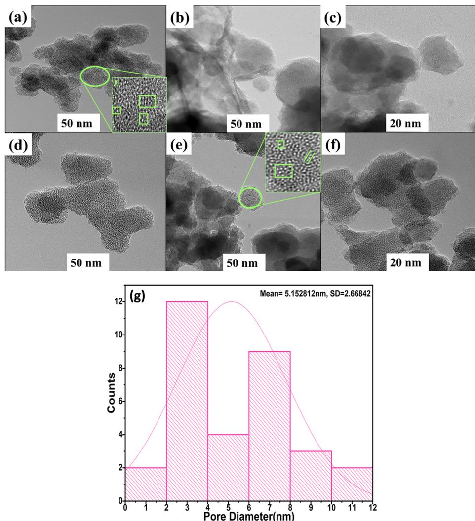
Fig. 10 HRTEM images showing the uniform pore channels of (a)–(c) MCM-48 and (d)–(f) SnO<sub>2</sub>/MCM-48(5%). (g) Pore-size distribution of SnO<sub>2</sub>/MCM-48(5%).
