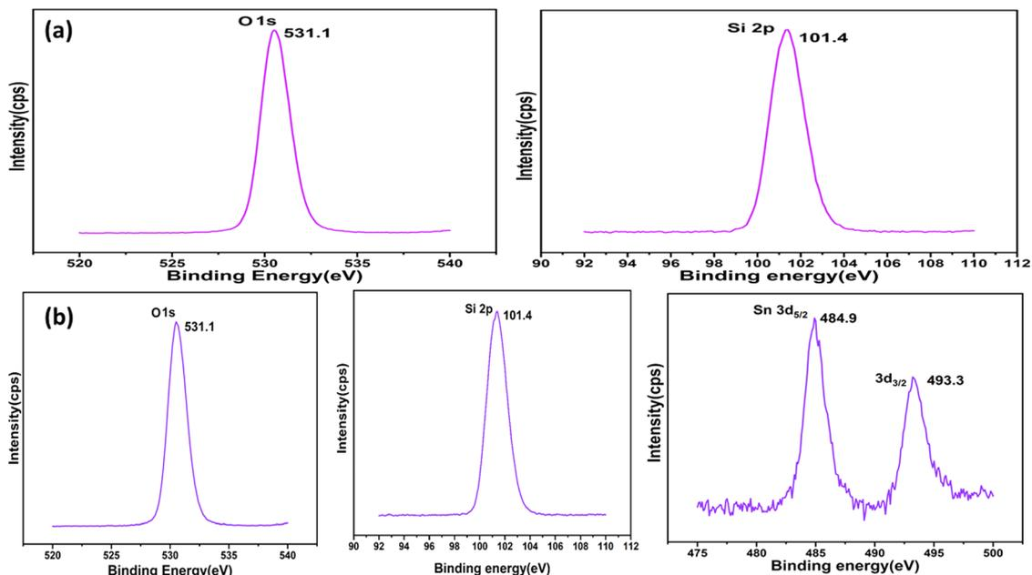
Fig. 8 XPS analysis of (a) MCM-48 and (b) SnO<sub>2</sub>/MCM-48(5%).
