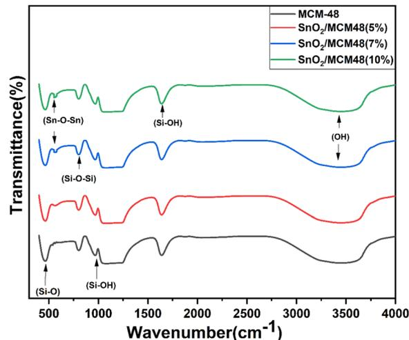
Fig. 7 FTIR spectra of MCM-48 and SnO<sub>2</sub>/MCM-48.
