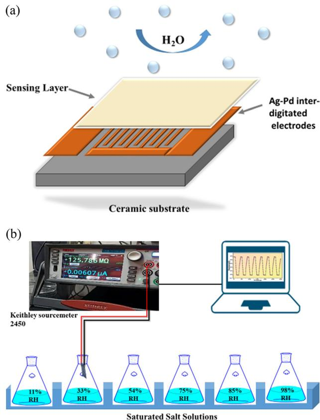
Fig. 2 (a) Fabrication of the humidity sensor. (b) Schematic illustrating the configuration of the humidity sensing set-up.
