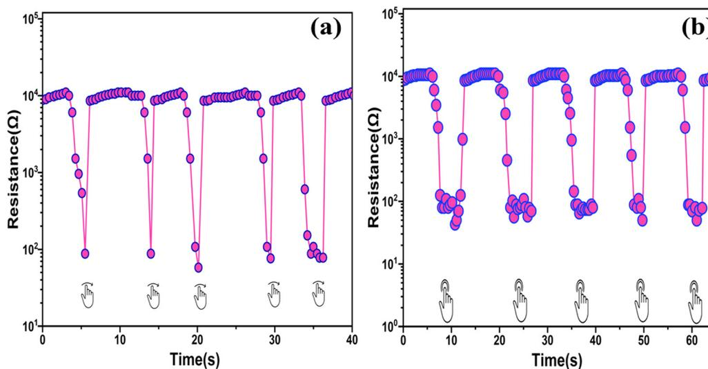
Fig. 19 Response of the SnO<sub>2</sub>/MCM-48(5%) humidity sensor to a (a) finger sliding over and (b) finger moving in an upward and downward motion at a distance of ~6 mm.
