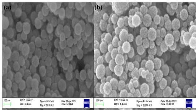
Fig. 5 FESEM images illustrating the morphologies of (a) MCM-48 and (b) SnO<sub>2</sub>/MCM-48(5%) at a scale of 100 nm.
