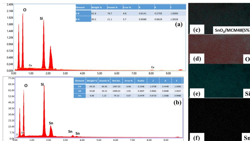
Fig. 6 EDX analysis spectra of (a) MCM-48 and (b) SnO<sub>2</sub>/MCM-48(5%). (c)–(f) EDX elemental mapping.
