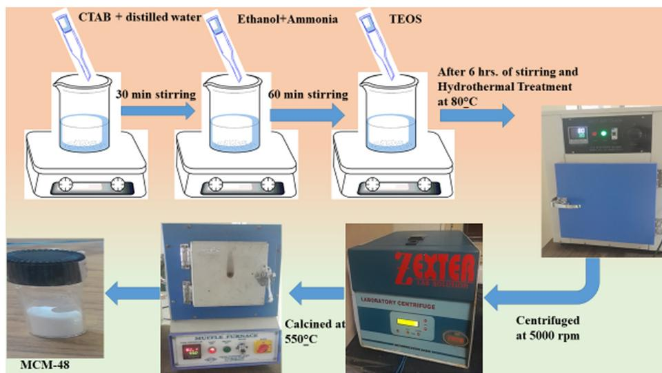
Fig. 1 Schematic representation of MCM-48's synthesis route.
