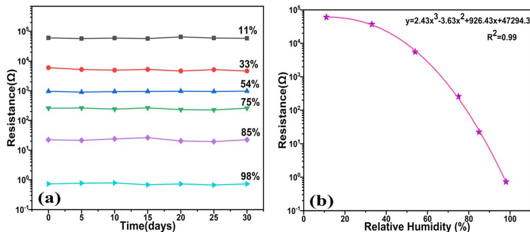
Fig. 15 (a) Stability plot of the sensor over a duration of 30 days. (b) Cubic polynomial fitting of the resistance with the RH%.
