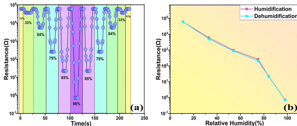
Fig. 14 (a) Uplink and downlink testing of the SnO<sub>2</sub>/MCM-48(5%) sensor. (b) Hysteresis characteristics of the SnO<sub>2</sub>/MCM-48(5%) sensor at varying RH (11–98%).
