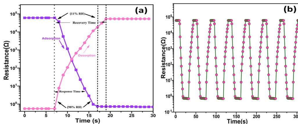
Fig. 12 (a) Response/recovery times for SnO<sub>2</sub>/MCM-48(5%); (b) response/recovery times for repeated cycles.
