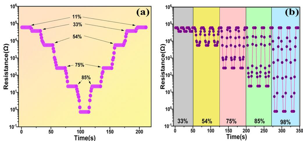
Fig. 13 (a) Staircase plot representation of the variation of resistance with time for the SnO<sub>2</sub>/MCM-48(5%) sensor. (b) Repeatability performance of the SnO<sub>2</sub>/MCM-48(5%) sensor exposed to 33% RH, 54% RH, 75% RH, 85% RH, 98% RH.
