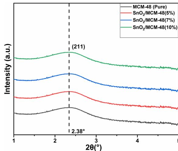
Fig. 3 Small-angle X-ray plots for MCM-48 and SnO<sub>2</sub>/MCM-48.
