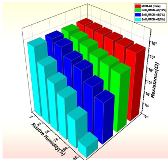
Fig. 11 3D representation of the change in resistance with respect to the RH% for MCM-48 and SnO<sub>2</sub>/MCM-48 nanocomposites.
