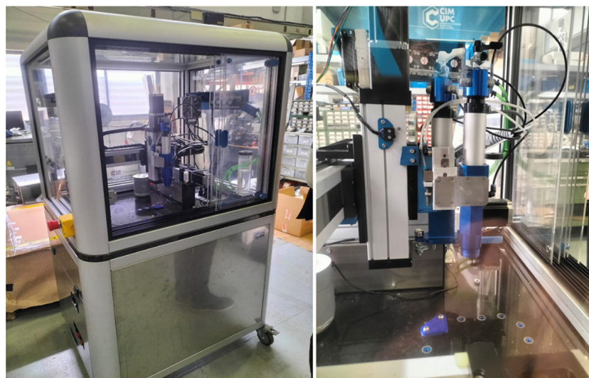
Fig. 1 PowerDIW 3D printer by CIM UPC. Details of the 3D printing moving part, DIW extrusion system and marble platform.
