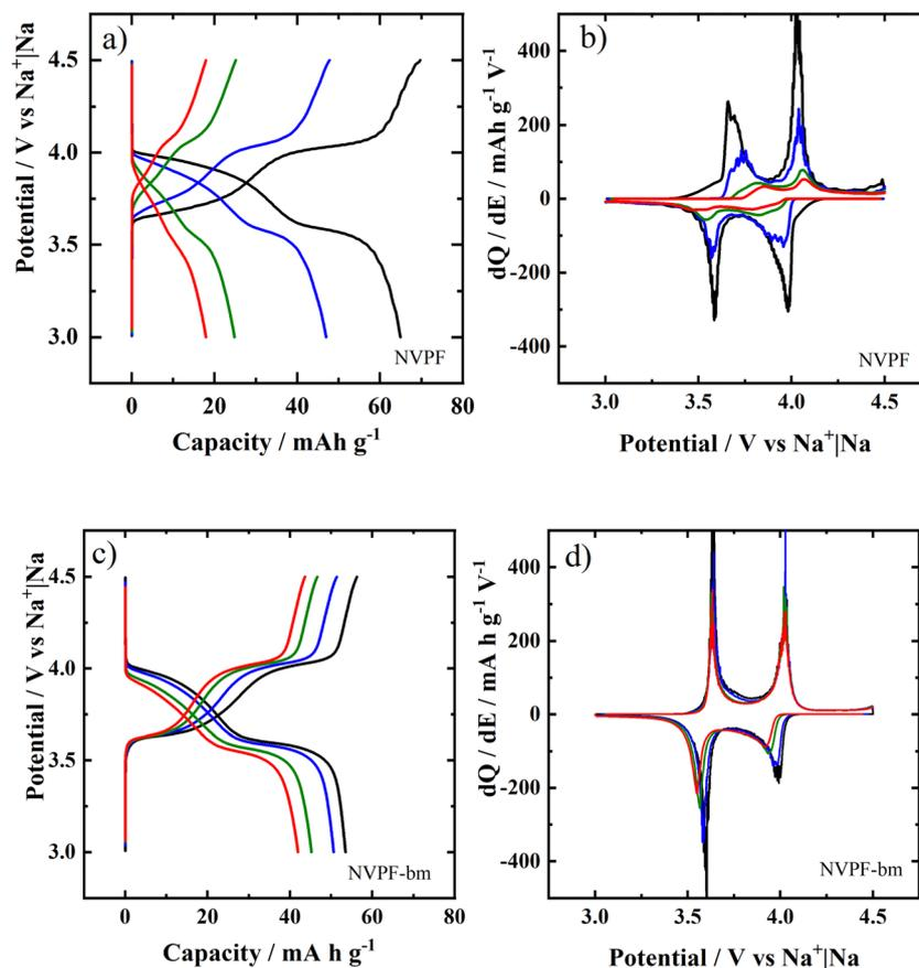
Fig. 3 Charge and discharge curves (10th cycle) and  $dQ/dE$  plots as a function of the potential of the NVPF (a) and (b) and NVPF-bm (c) and (d) electrodes at 0.01 (—), 0.02 (—), 0.05 (—) and 0.07 (—)  $A g^{-1}$ .
