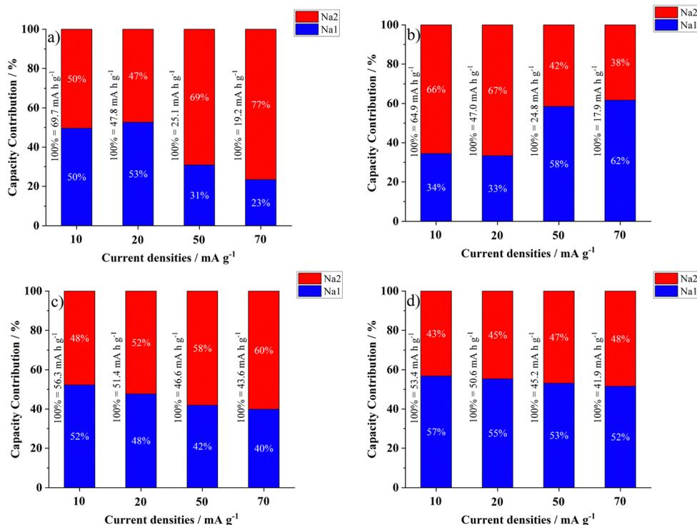
Fig. 4 Capacity contributions of (blue) Na<sup>+</sup><sub>1</sub> and (red) Na<sup>+</sup><sub>2</sub> to the (a) and (c) charge and (b) and (d) discharge processes of the (a) and (b) NVPF and (c) and (d) NVPF-bm electrodes.
