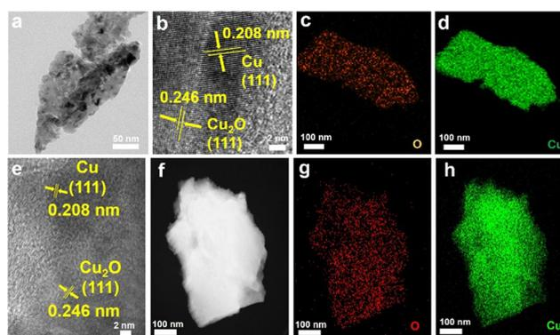
Fig. 2 TEM images (a), (b), and (e), HAADF-TEM (f), and elemental mappings (c), (d), (g), and (h) of the CC@Cu<sub>x</sub>O (a)–(d) and CC@Cu<sub>y</sub>O (e)–(h) samples.
