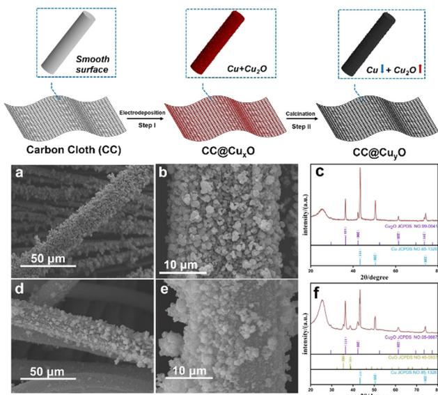
Fig. 1 Schematic illustration of the synthetic process (top image), and SEM (a), (b), (d), and (e) and XRD patterns (c) and (f) of the CC@Cu<sub>x</sub>O (a)–(c) and CC@Cu<sub>y</sub>O (d)–(f) samples.
